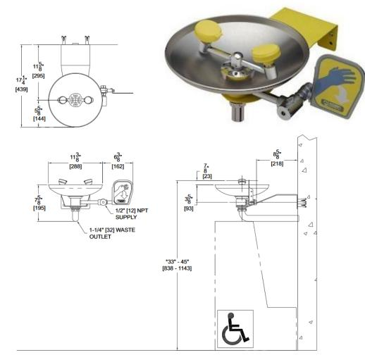
Model S0440-BF is our wall mounted DDA compliant stainless steel eye/face wash complete with stainless steel bowl and yellow coated galvanised steel mounting bracket. Comes complete with plastic eye/face wash spray heads, an inline strainer and a stay-open 1/2" ball valve with a push handle. Barrier free, suitable for wheelchair users. Compliant to ANSI Z358.1 standards, including a safety sign and weekly testing card.
